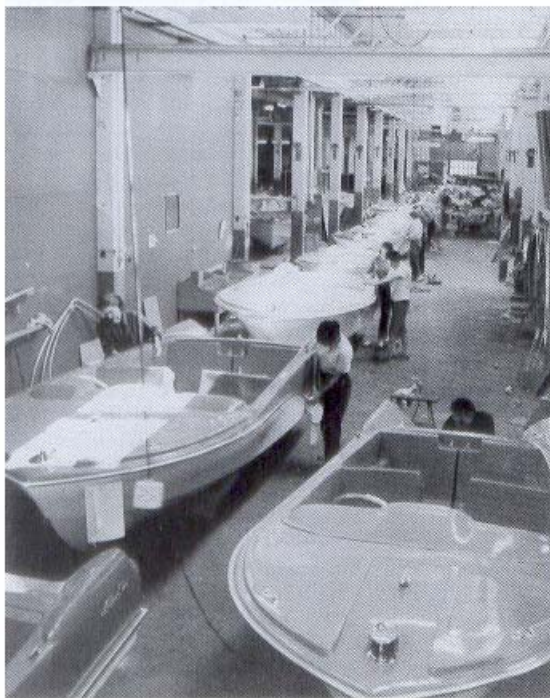
Lake 'N Sea boats receive trim and hardware at the Michigan Fiberglass Plastics plant.
